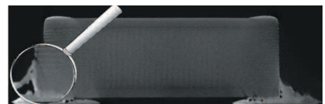
Ceramic resistance defects: • crack on substrate • delamination on terminations
